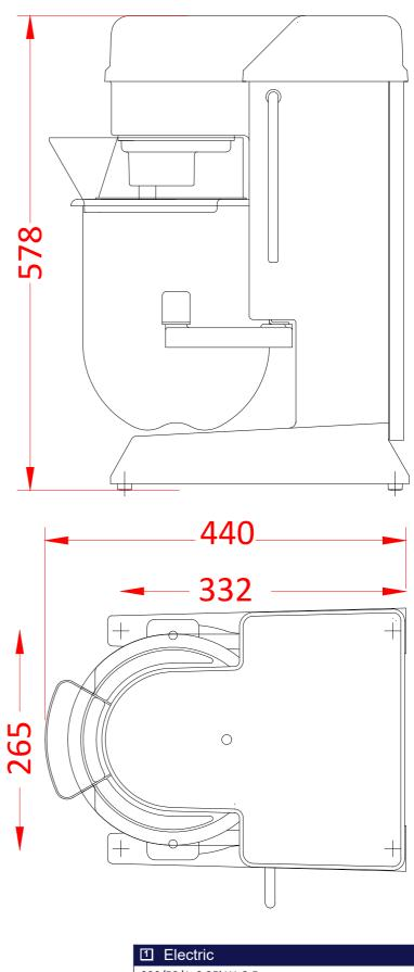
230/50/1 0.35kW 3.5amps MIXER COMES WITH 13amp PLUG FITTED WITH 13amp FUSE.
